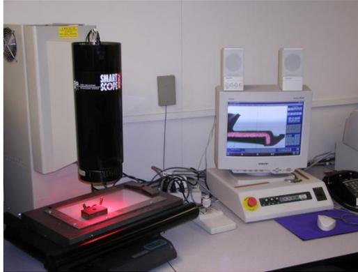
Smart Scope used in non-contact measurement of seal geometry. Typical measurements of radial and axial lip heights and diameters are gathered here.
