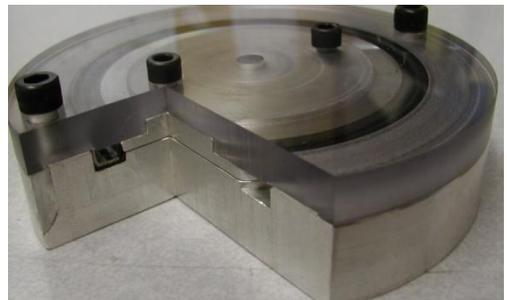
Design fixture used to simulate the interference fits while seeing the effects on axial and radial lips. Cross sectional and top views of the seal lips visible.
