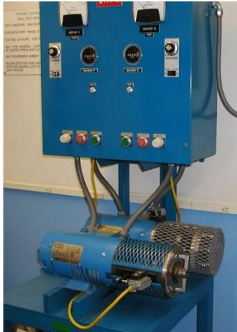
Test heads used for seal only testing. Seals are tested until failure.
