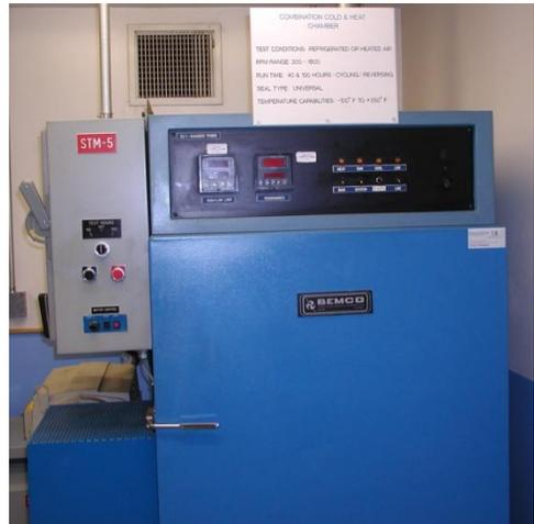
Temperature test chamber capable of -100 F to +350 F. Rotation of a shaft is performed by a side mounted motor for seal testing.
