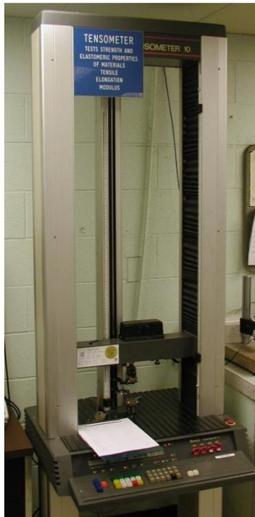
Tensometer used to determine physical properties of rubber compounds (Tensile, Elongation and Modulus).
