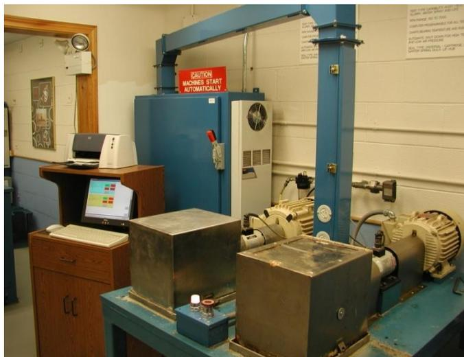
Additional test rigs for seal testing. These are specifically designed for mud spray and submersion tests. These rigs are used with the bearing to conduct the test. Similar controls and measurements performed on these rigs.
