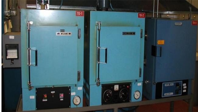
Lab ovens used for grease compatibility trials, heat aging, post cure of test slabs, compression set trials. These trials can last up to 42 days at elevated temperature. Ovens capable of 500 F.
