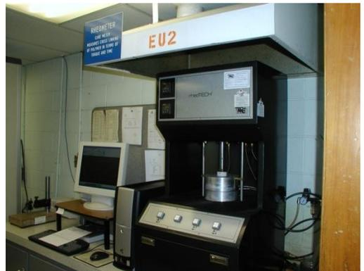
Rheometer used in the evaluation of rubber compounds. Determines the rate of cure and how the compound will process. Useful in setting up new manufacturing cycles.
